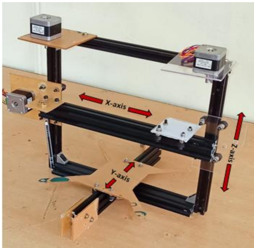
Fig: 5.3: Representing X, Y and Z axes in 3D Printer.
